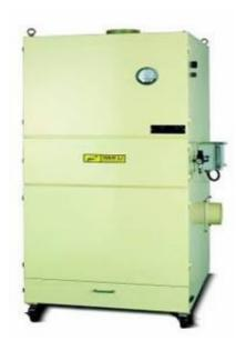
The exhauster blower cleans the dust-loaded air out of the tablet bed by blowing it throughout the exhaust filter. A temperature sensor controls the exhausted air.
