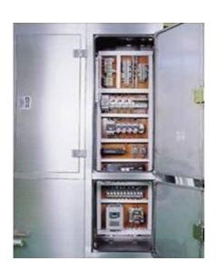
The terminal box is integrated into the housing of the coating unit. All electrical parts of the control system are within there.
