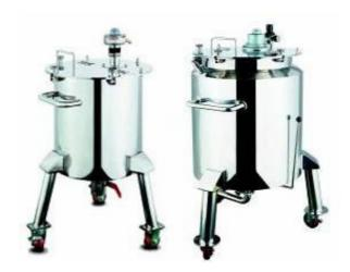
There are two different tanks for film and sugar coating solutions.
